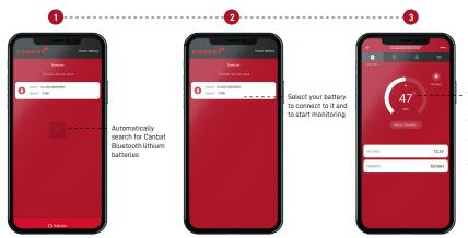
This is the main dashboard. From this screen, you will be able to monitor the state of charge (SOC), battery's status, battery's health, voltage and Capacity
